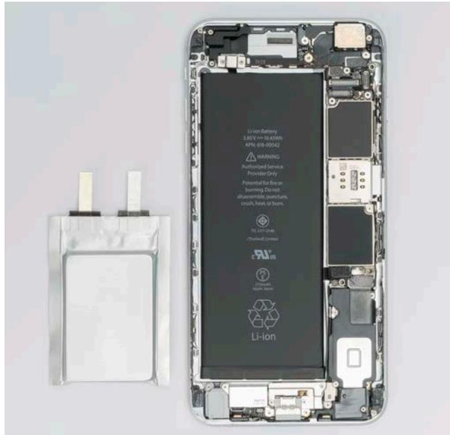
**Figure 4 | Half the size and half the weight.** A SolidEnergy 3Ah cell (left) in comparison with an iPhone 6 Plus 3Ah cell (right).
